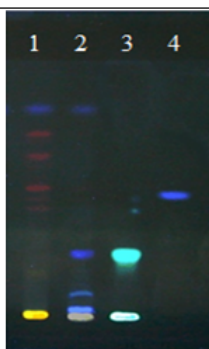
Fig. 4 Chromatogram obtained after spots visualization with DFBOA, (mobile phase B) 1. TPF; 2. M-fr; 3. chlorogenic acid; =4. ferulic acid.
